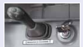
Dozer float function and travel mode switch
